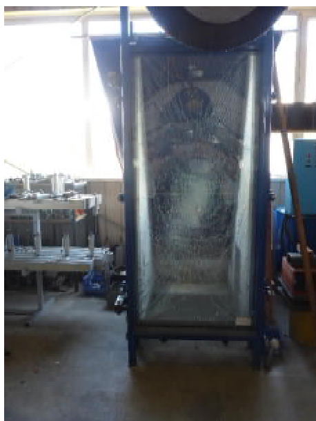
Fig. 2: Test specimen 55 with fracture behaviour of type B
