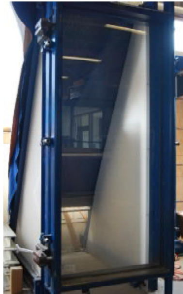
Fig. 1: Pendulum test stand with test specimen
