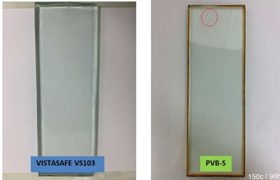
Picture 3. Samples of laminated glass of VISTASAFE VS103 vs PVB-S [66.4]
